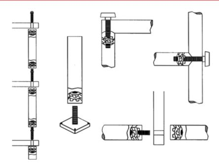
Inside Tube Diameter = 24,6-25,6Outer tube diameter = 1 1/8" Thread = M 10
